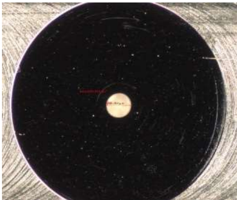
Figure 24 – An optical image of the diamond turned surface around the cavity. The black is a highly reflective surface that is not scattering the light from the microscope.
