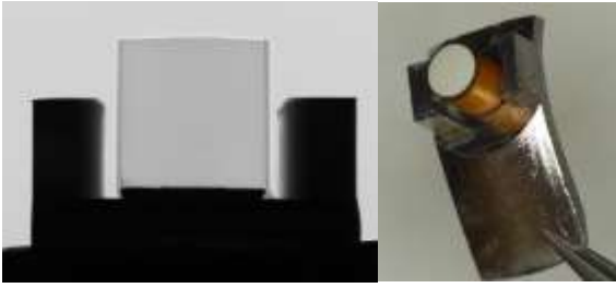
Figure 16 – a) Left - x-ray radiography showing the foam quality of a completed target. b) Right - optical image of the complete target.
