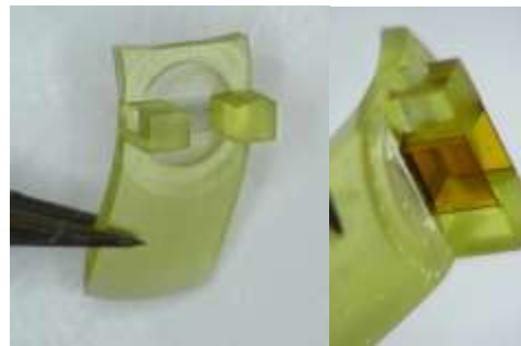
Figure 9 – Optical images of a 3D printed clip holder. a) Left - without the PI windows. b) Right - with additional assembly of PI windows.
