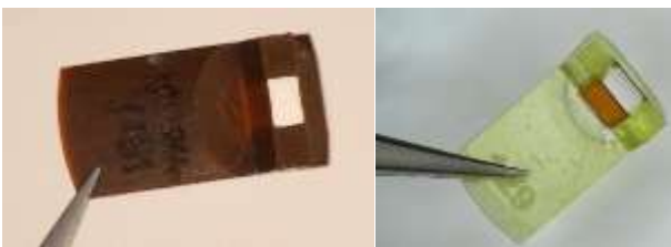
Figure 13 – Optical images of the complete target as seen from above. a) Left - in a Vespel holder and b) Right - in the 3D printed holder with additional PI windows.
