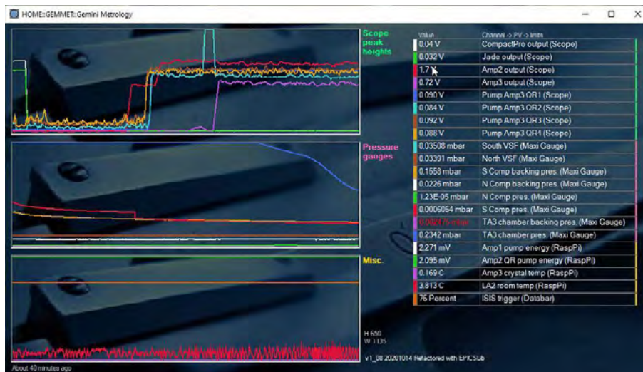
The Gemini Metrology application (formerly Mon&Cont). There was a spike on Amp3 output as the system was brought up, the TA3 Target Chamber is being pumped-down, and the ISIS trigger is holding steady.
