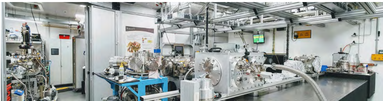
Figure 3: User area in the new laboratory. The beamline closest to the camera is the flat-field imaging beamline; the beamline behind it is for photoemission spectroscopy from the gas phase (see the chamber on a blue table-frame, docked at the beamline's end). At the back of the lab, behind the partition, are beamlines for solid-state photoemission (the material science chamber is just visible at left) and – not visible here – a beamline for infrared spectroscopy.
