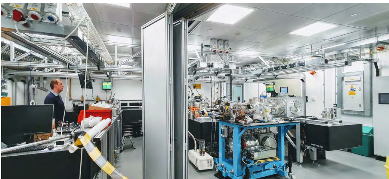
Figure 4: Another view of the lab. A partition, at centre, allows the lab to be divided into two separate rooms. The beamline at left is the solid-state photoemission beamline, under construction. Just to the right of the partition is the beamline for photoemission from the gas phase. At far right is the flat-field imaging beamline.
