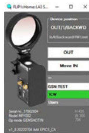
Figure 3: Flipper control interface configured to move a flipper into the alignment section of the beamline on-shot, to block back-reflections from the full power section.
