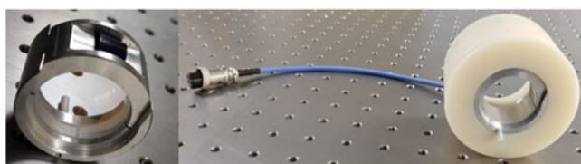
Figure 3: Photographs of LBO crystal oven components: (left) spring-loaded metallic crystal holder with the crystal in place. This is placed inside the oven unit (right). The oven is then connected to a separate temperature control unit.
