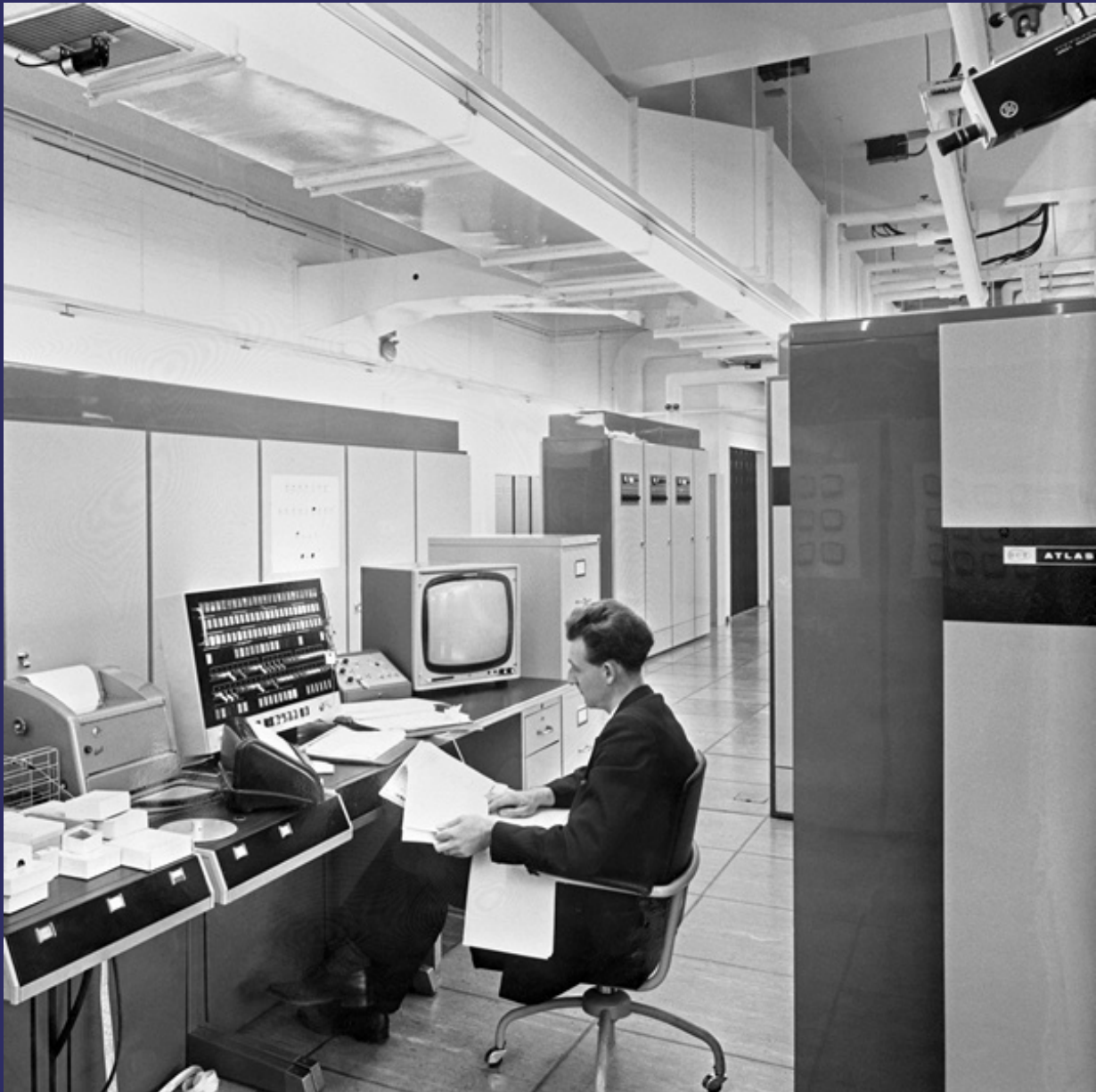
Ferranti/ICT engineer David Burrell at the Engineer's Console of the Atlas computer in the Atlas Computer Laboratory machine room. (1968)
