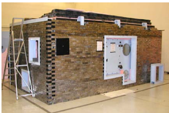
Figure 1. Lead shielding surrounding the PW chamber required for high atomic number target experimental investigations.
