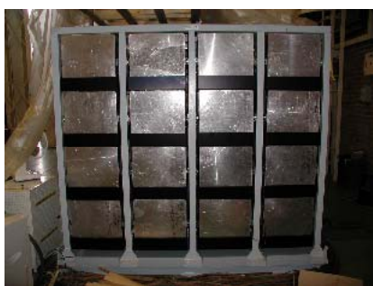
Figure 1. One of the two LaNSA array for PW experiments, which consists of 16 modules, each of which includes 16 scintillator / PMT detectors, corresponding to 256 detectors.
