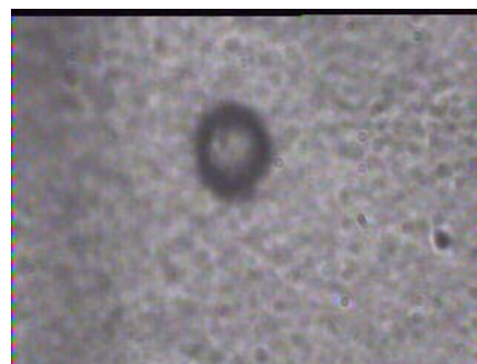
Figure 2 . Preliminary Image of UV 'ring', reduced by 100x, produced in homogeneous Gafchromic film – the outer ring is 10µm in diameter and 1.2µm in width.
