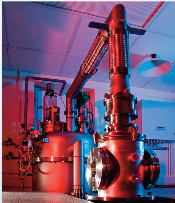
DiPOLE prototype cryogenic amplifier with cooling system in background.
