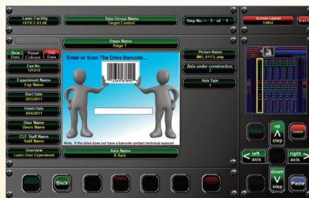
Drive System Editor which aids experimental setup and drive connections.
