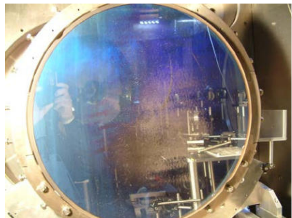
Figure 4: Damage across half the beam area of the protective overcoat on the silver coated final focusing parabola
