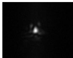
Figure 1b image of focus corrected. Spot is 23\mu\text{m} FWHM, 1.25x diffraction limited
