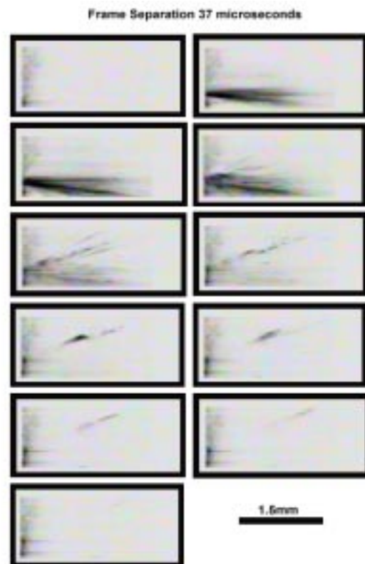
Figure 2. Melt ejection filmed at 27,000 frames/s.
