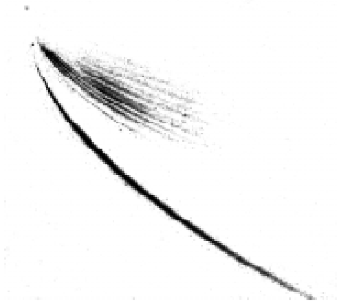
Figure 3. Raw data on a CR39 track detector from an aluminium target. A single proton parabola and many parabolas from different charge states of aluminium ions can be observed. All the parabolas have their origin on the mark left by neutral particles in the top left corner
