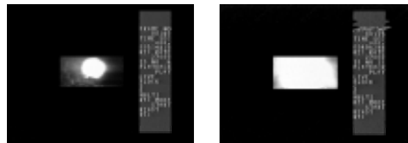
Figure 6. Images of the plasma plume at its maximum size for 7.3 and 18 J pulses.
