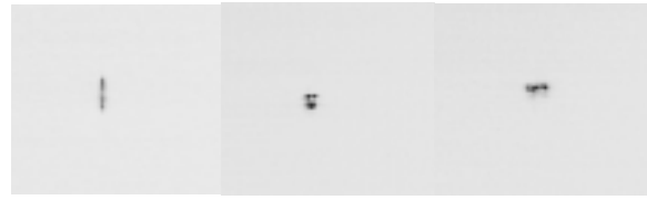
Figure 5. Focal Scans Showing Astigmatic Farfield.
