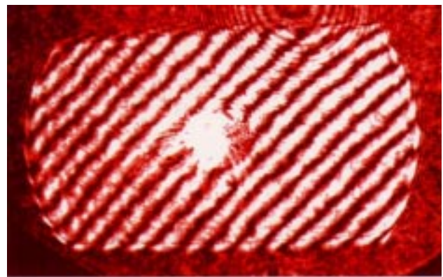
Figure 1. Interferogram showing the wavefront accuracy of the parabola in double pass at 633 nm.
