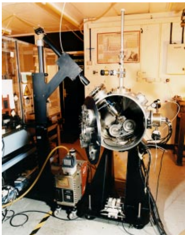
Figure 2. Photograph of soft X-ray source used at the Rutherford Appleton Laboratory.
