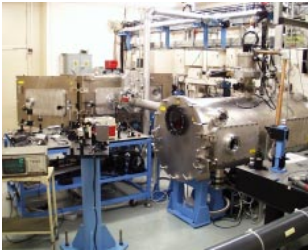
Figure 5. Target Area 2 showing the compressor chamber (foreground) and target chamber.
