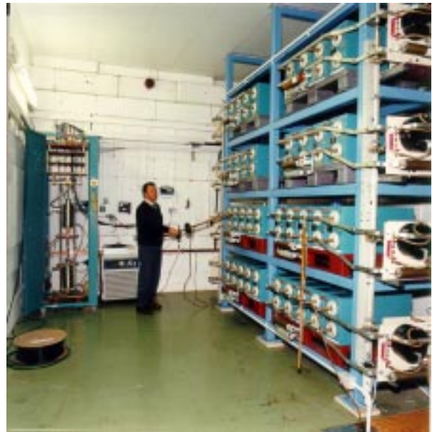
Figure 1. Pulsed power test bank assembled using NOVA components.
