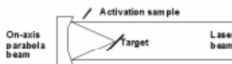
Figure 1. Schematic experimental lay-out. Laser beam entering from right is focused by an on-axis parabola (left) to target surface (middle). Blow-off plasma hits activation sample (top) in the target normal direction.
