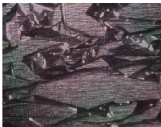
Figure 2. Iron substrate with Manganese deposition.
