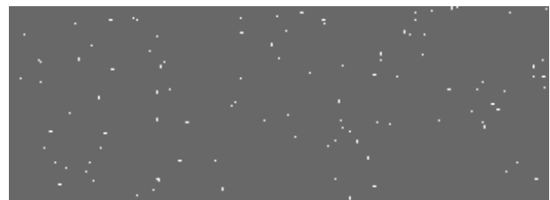
Figure 2. A typical image from the Ti target taken with the Andor technology CCD camera filtered with 25 \mu\text{m} Be, 23 \mu\text{m} Mylar, 25 \mu\text{m} Teflon, 10 \mu\text{m} Cu, and 10 \mu\text{m} Ti. The probability of finding two or more photons in one pixel is low.
