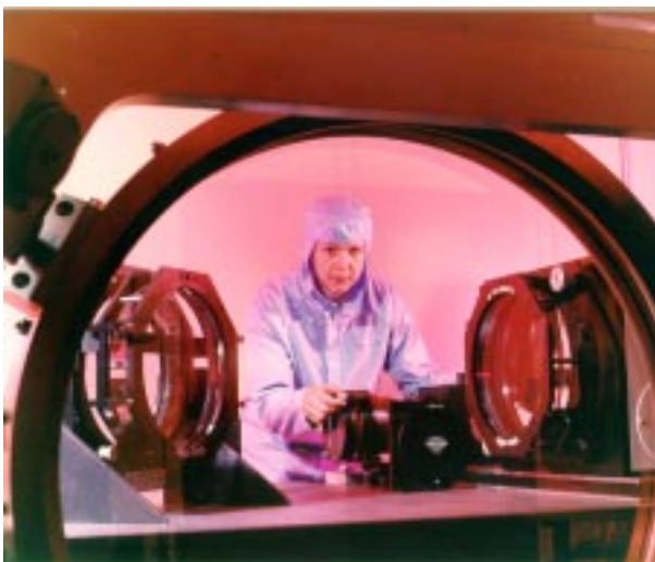
Figure 2. Placement student Keith Hughes adjusts the interferometer arrangement, with a 940 mm diameter mirror from the Vulcan Petawatt Upgrade in the foreground.
