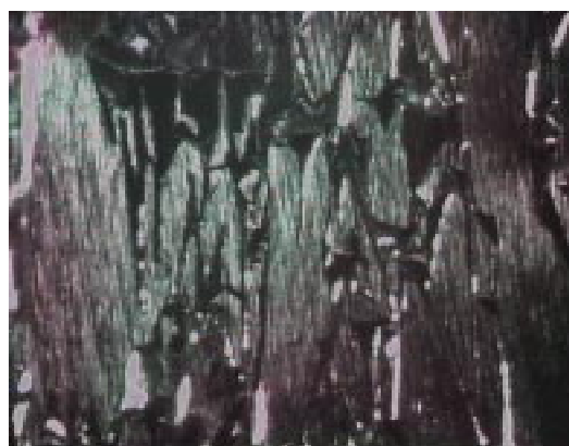
Figure 3. Copper substrate with Manganese deposition.
