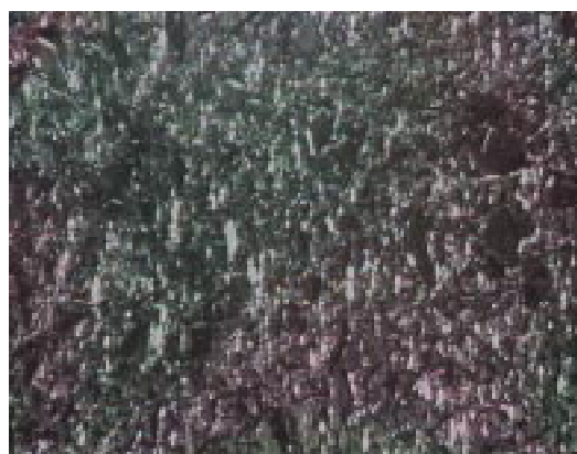
Figure 1. Aluminium substrate with Manganese deposition.
