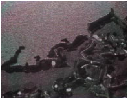
Figure 5. Stainless steel substrate with Manganese deposition.
