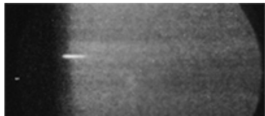
Figure 3. The 3ps x-ray laser observed using the femtosecond x-ray streak camera.
